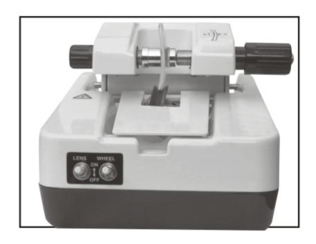
3.turn on the lens rotating switch, put the head down. Make sure that the lens locates well.
