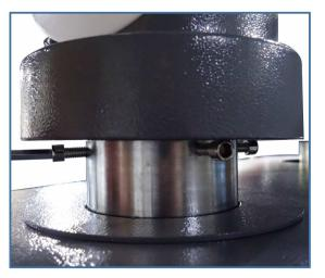
8. Put the big table-top above the main machine, and insert the two cables into the bearing hole (as shown in the figure below).
