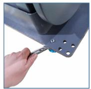
4. Take out the pedal support, assemble the inner hexagon screws (M8\*4pcs) in the corresponding holes, adjust the height of pedal pad if the ground is not flat.
