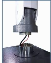
7. Adjust the direction of the phoroptor arm to be perpendicular to the main machine, use an Allen key to lock the screw which are inside the arm.
